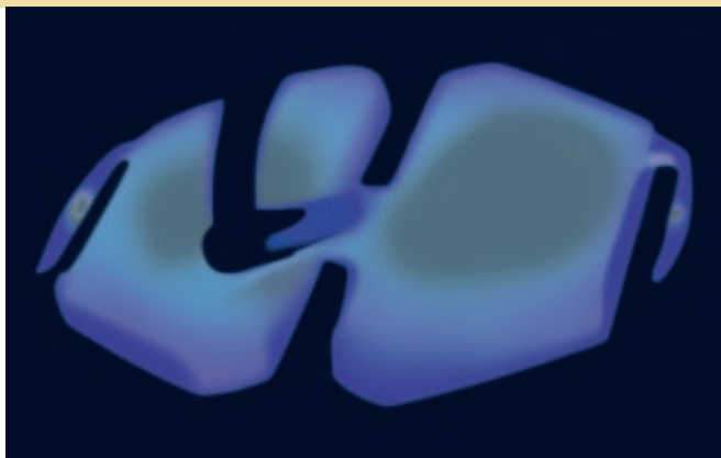
Heat distribution on surface of light head housing.
